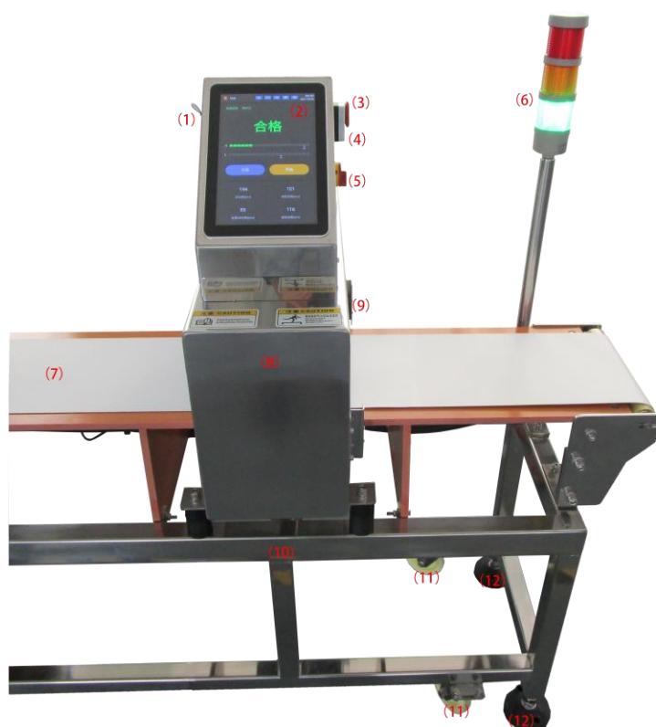
Figure 2-1 Metal detector machine structure diagram
