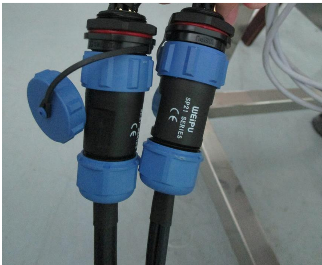
Figure 2-5 Connect the rejector part to the electrical box
