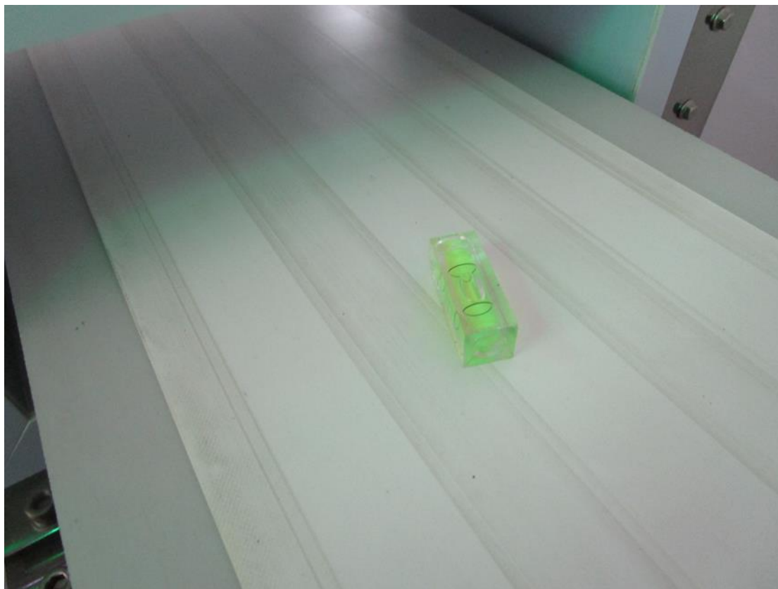
Figure 2-3 Determine whether the conveying surface is level by the bubble level
